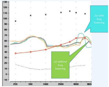
To adjust frequency lowering settings to maximize audibility, filtered 6400 Hz speech stimuli to stimulate /s/ is used to maximize the amount of energy above the child's audiogram with the minimum amount of lowering of frequency. The green line represents the verification of the 6300 Hz /s/ stimulus without frequency lowering and the aqua line represents verification of 6300 Hz /s/ with frequency lowering activated on the HA.
